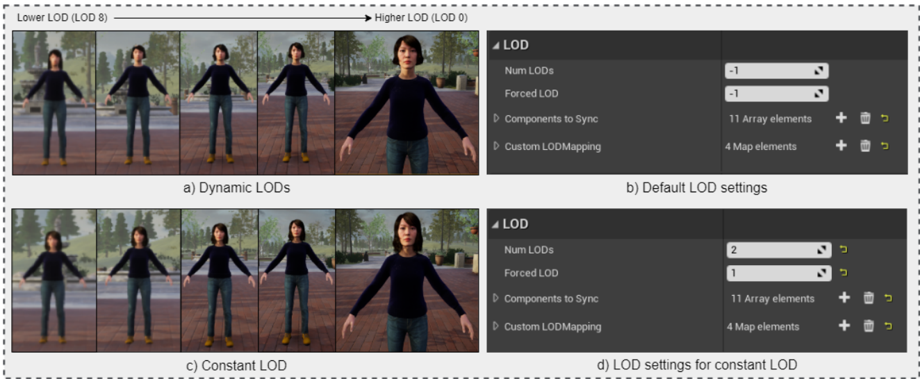
Figure 4. Dynamic LODs vs Constant LOD . a) The Dynamic LOD system loads different meshes with various level of details based on the proximity to camera. This however results in sudden popping up of the meshes which generates artefacts in the data. b) Default LOD settings used by the engine. c) The modified LOD system is used to maintain LODs at a fixed LOD so that the avatar’s appearance is unaffected by distance. d) The LOD of the character is locked to 1 using Forced LOD.
